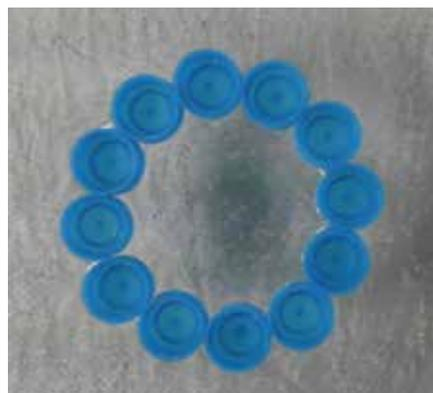
Circle of caps behaves as a rigid object: wind takes it without deforming it, and waves at the water surface do not modify its shape
